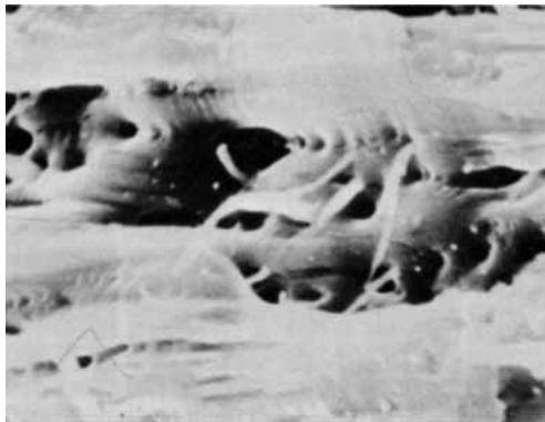
Fig. 25. Axial split interface of an EDBH fiber fractured at 65% RH. Cortical cells seem to have been torn apart (6500 \times ).
